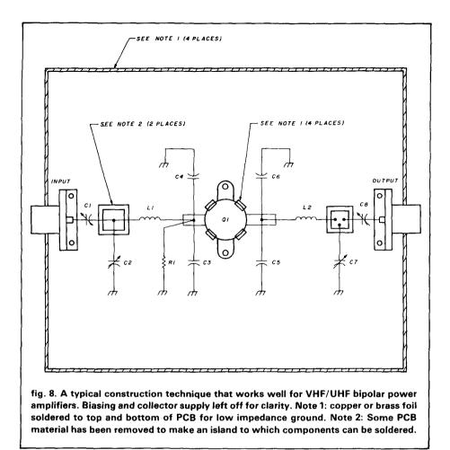
shot design that is unproven, the discrete inductor is hard to beat. If you err in the value, just add a turn to or drop a turn from the coil and you're back in business. It isn't easy to cut up, extend, or decrease the length of a microstrip line on a printed circuit board if the tuning is incorrect!
